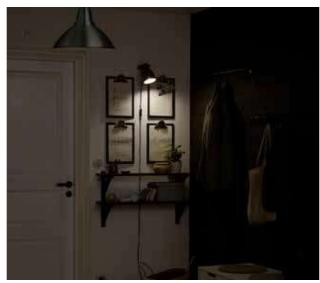
Choose a location to install your motion sensor. It has a maximum range of 10 metres to the light source (not blocked by walls), and a motion-reaction range of 5 metres and a 120° angle.
