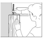
Place the newly cut edge of the filler piece against the wall (it should fit perfectly). Mark the edge of the cabinet on the top and bottom of the filler piece. Draw a straight line from these points and cut.
