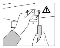
Install your lighting and appliances. If drilling holes, use a piece of wood to meet the drill as it penetrates the surface to avoid the edges from splintering.
