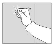
Check your wall is strong enough to hang your suspension rail and cabinets. Depending on your wall material, it's best to install your rail onto a stud or a support beam. An electronic stud finder can be helpful.
