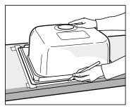
Mark a spot for the sink by laying the worktop in place. Trace the inside of the base cabinet onto the underside of the worktop. This helps you align your sink. Turn your worktop over and trace the outline of your sink onto masking tape.
