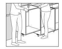
Cabinet legs connecting two cabinets can be used to support both cabinets while you're installing. Remember to use the distance ring included with the legs.
