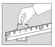
If your wall is uneven use distances between the rail and the wall to make sure the rail is straight.
